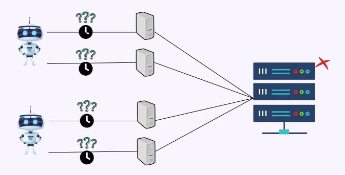
Attack in which the attacker exploits publically-accessible Network Time Protocol (NTP) servers to overwhelm the targeted with User Datagram Protocol (UDP) traffic.
