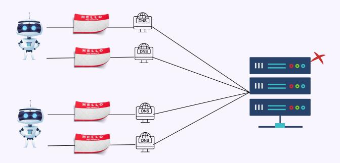
Attack in which the attacker exploits vulnerabilities in domain name system (DNS) servers to turn initially small queries into much larger payloads, which are used to bring down the victim's servers.
