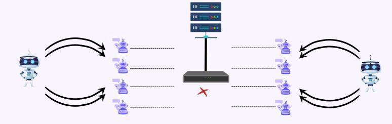
Attacker overwhelms random ports on the targeted host with IP packets containing UDP datagrams.
