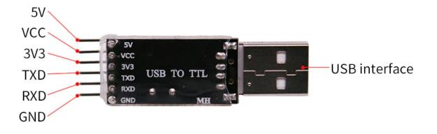
5V or 3V3 power supply can be selected by shorting circuit cap, The voltage selection of the short-circuit cap on the 6PIN pin Connect 5V-VCC short circuited to 3V3-TTL output Connect 3V3-VCC short circuited to 5V-TTL output.
